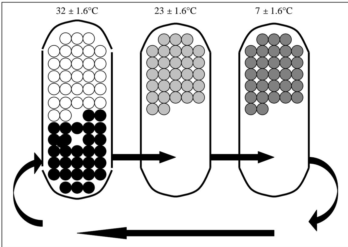
Figure 1. Schematic of Curing Tank Set-up and Rotation of Variable Cylinders
