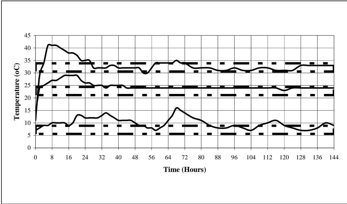
Figure 3. Temperature Logger Profiles for 32, 23, and 7° C Cylinders
