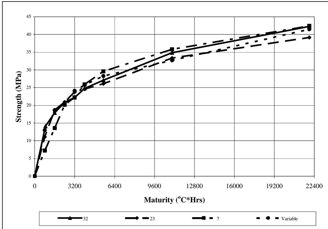
Figure 2. Compressive Strength vs. Maturity at Various Curing Temperatures
