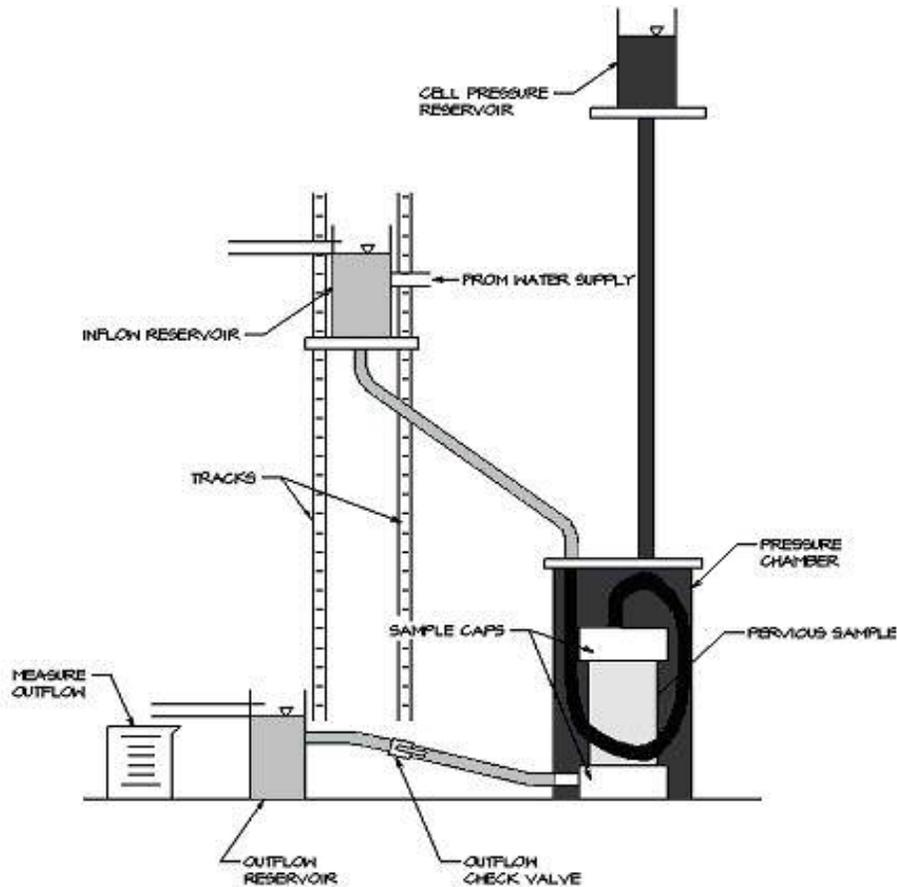
**FIGURE 1 Sketch of Simple Constant Head Triaxial Flexible-wall Permeameter**
