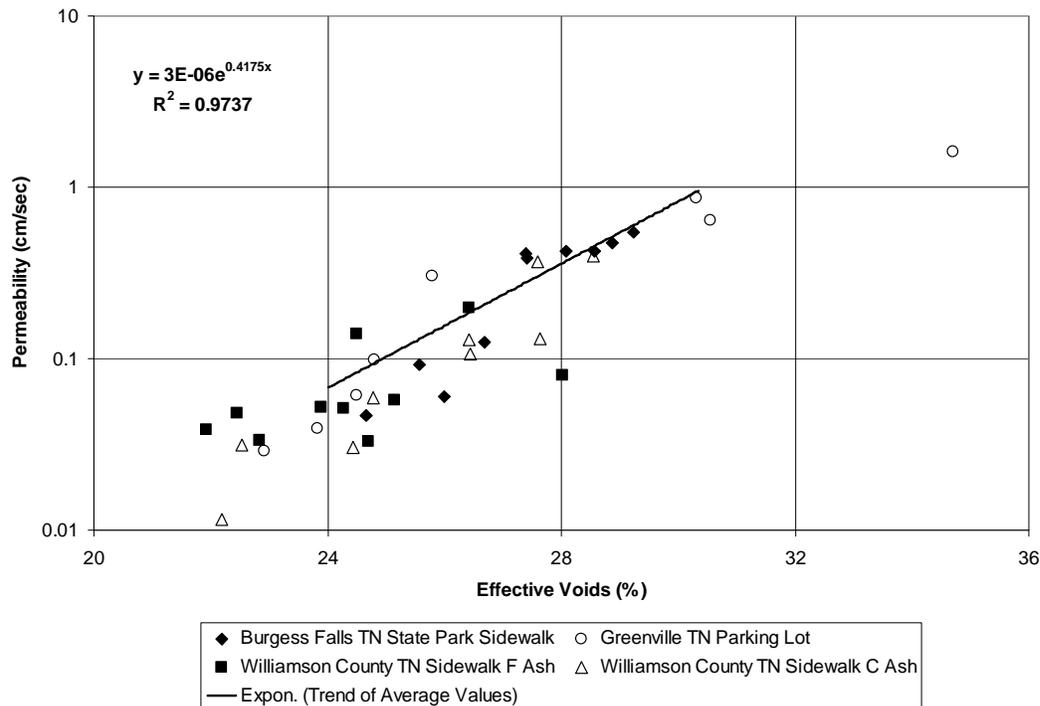
**FIGURE 4 Permeability vs. Effective Void Content for Cores from 2005 TCA Field Demonstrations**
