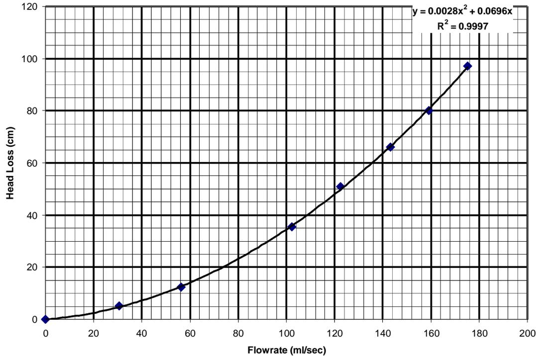
**FIGURE 2 Experimental Determination of System Head Loss.**
