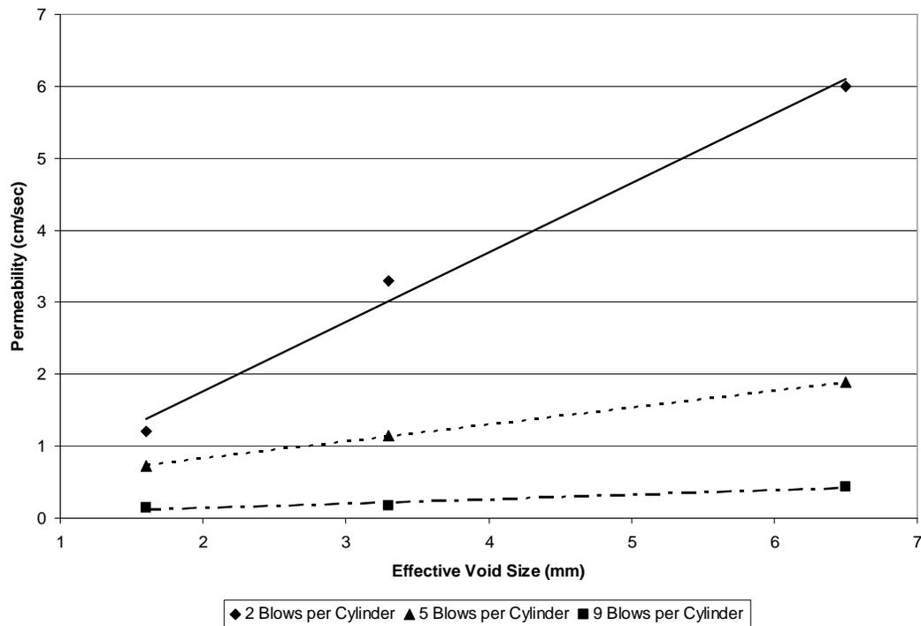
**FIGURE 5 The Effect of Void Size on the Permeability of Lightly Compacted Laboratory Limestone Aggregate Pervious PCC**
