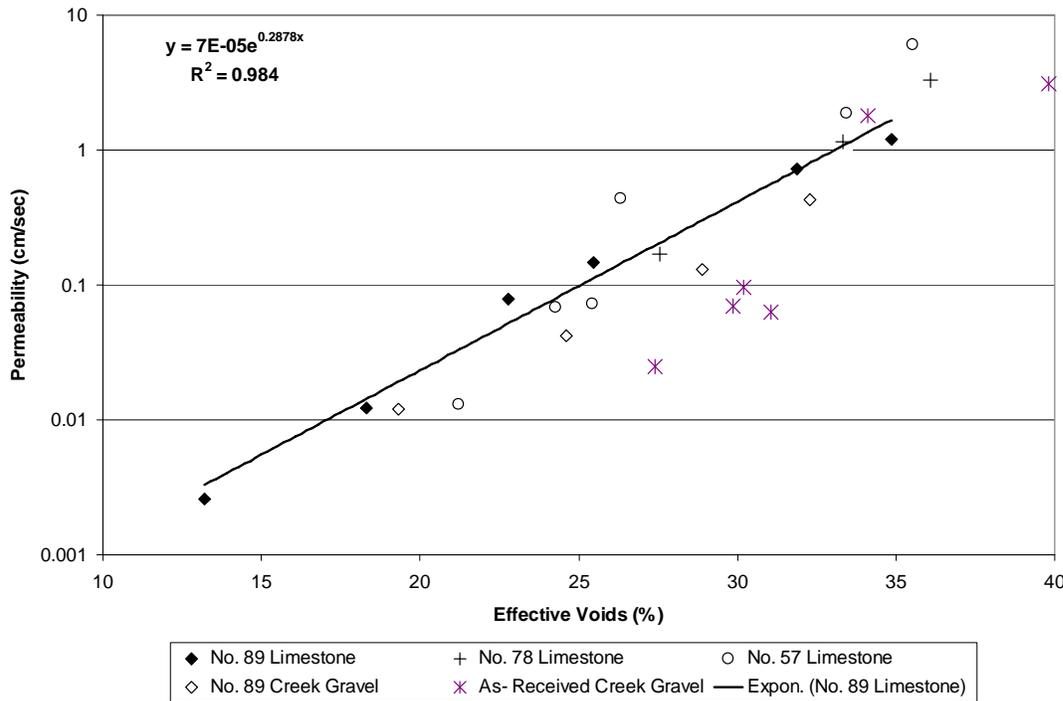
**FIGURE 3 Permeability vs. Effective Void Content for Laboratory Compacted Samples**
