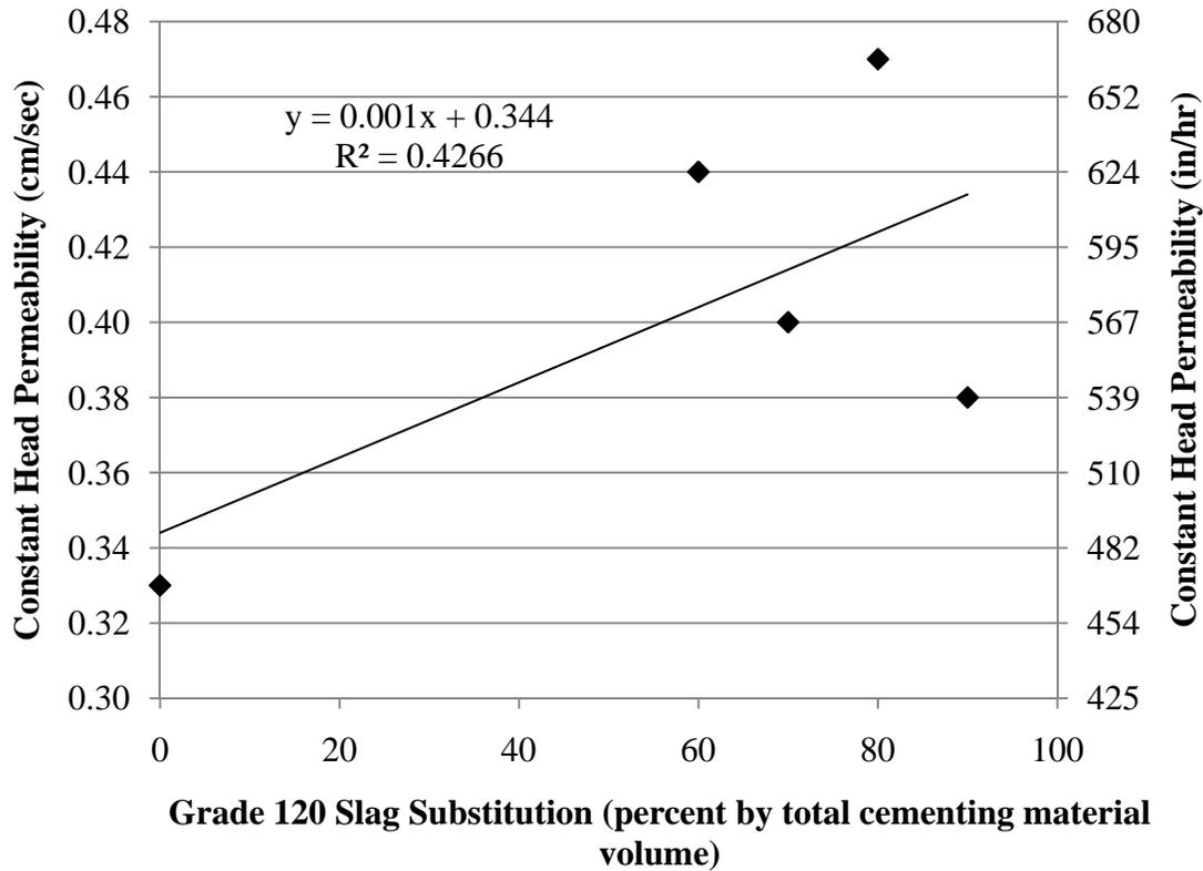
**Figure 2. Mean Constant Head Permeability versus Percent Grade 120 Slag Substitution**
