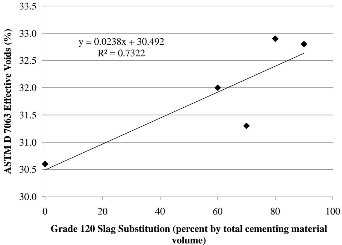
**Figure 1. Mean Effective Void Content versus Percent Grade 120 Slag Substitution**
