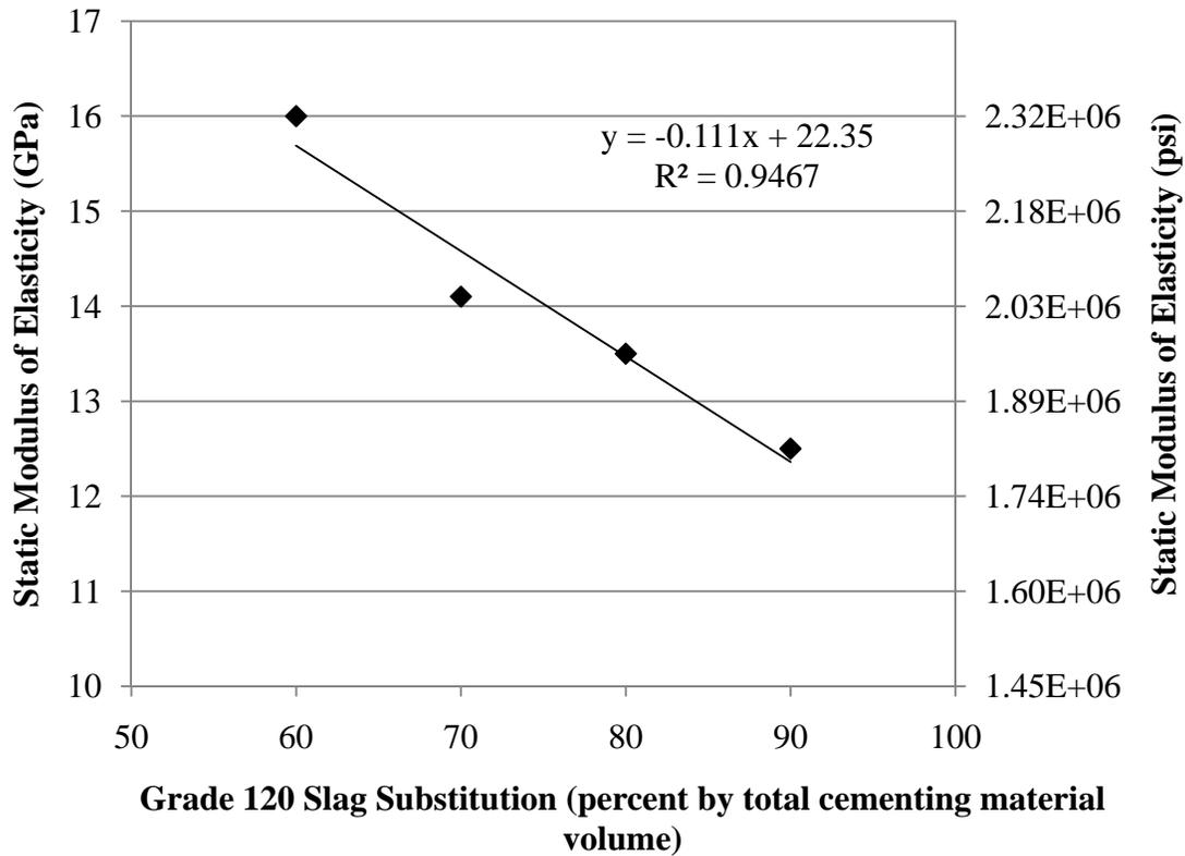
**Figure 4. Mean Static Modulus of Elasticity versus Percent Grade 120 Slag Substitution**
