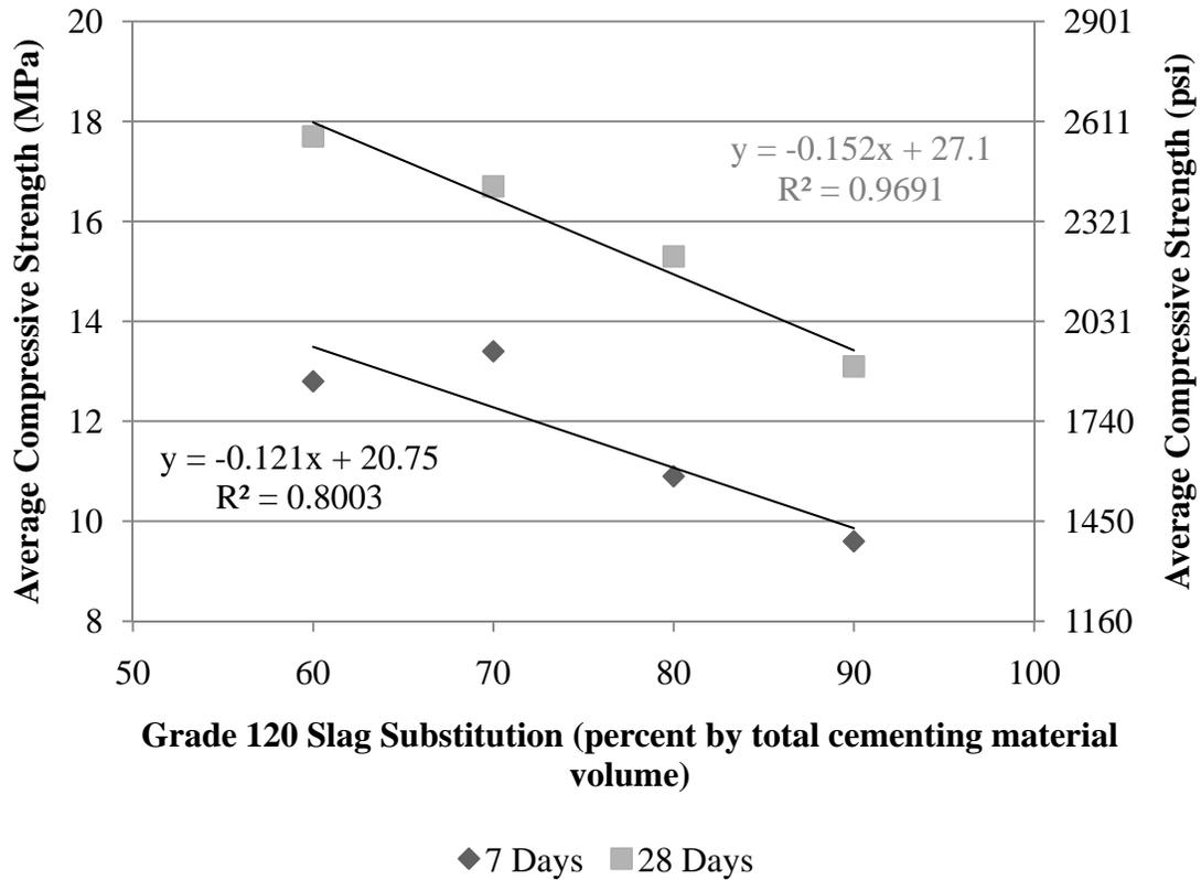
**Figure 3. Mean Compressive Strength versus Percent Grade 120 Slag Substitution**
